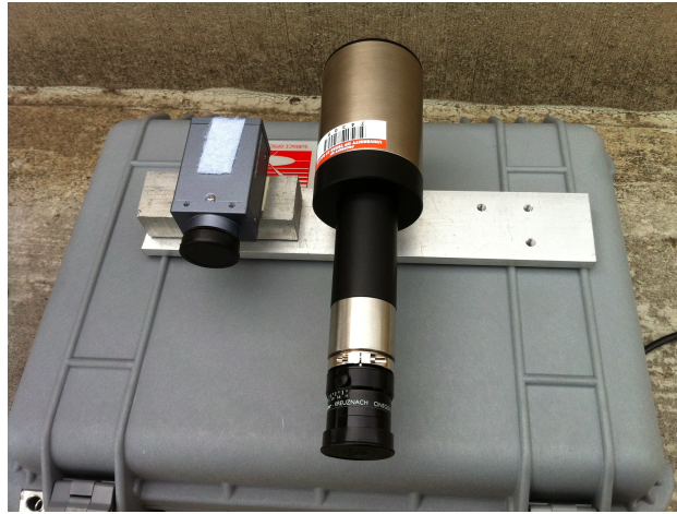
Figure 5. Experimental camera array. The hyperspectral camera has a cylindrical shape and it is shown in the middle, with the smaller conventional camera to its left.
